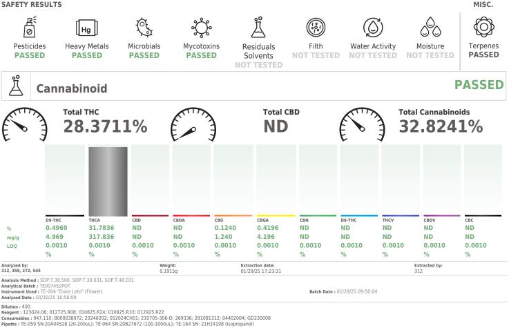
Fill spectrum cannabinoid analysis utilizing High Performance Liquid Chromatography with Photo Diode Array detector (HPLC-PDA) for analysis. (Methods: SOP.T.30.500 for sample homogenization, SOP.T.30.031 for sample prep, SOP.T.40.031 for analysis on Shimadzu LC-20X0 series HPLCs). Potency results for cannabis flower products are reported on an "as received" basis, without moisture correction.
